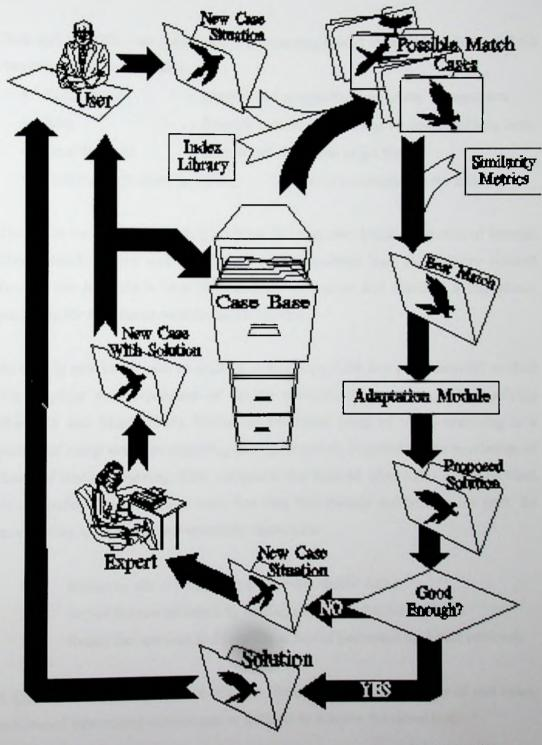
Fig 9. Data Flow of a CBR
