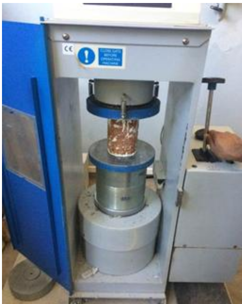
Figure 82: Checking the compressive strength of MC sample
