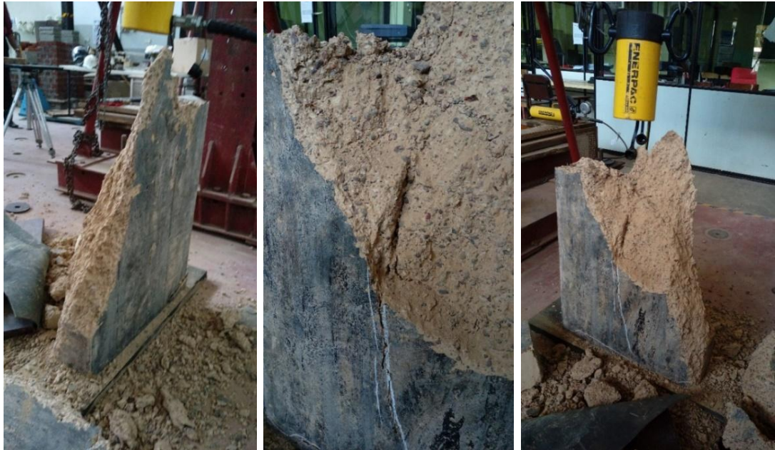
Figure 95: Observing the pattern of crack development between joints
