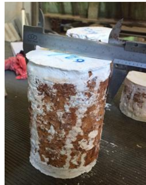
Figure 83: Applied capping on both side of MC sample
