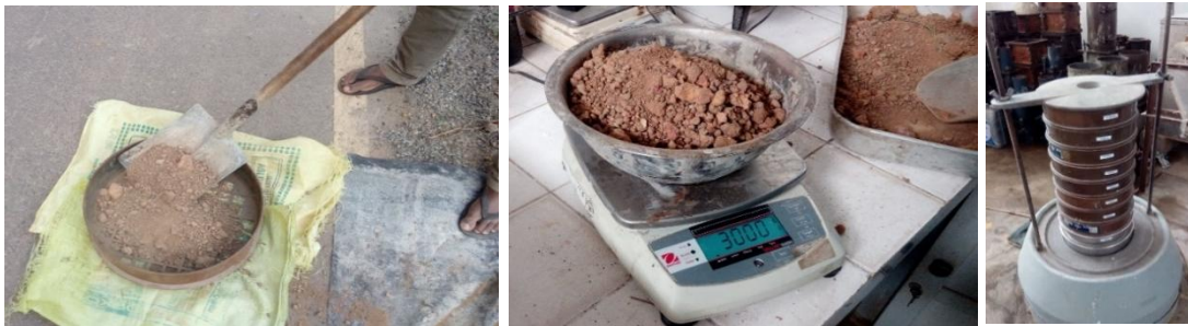
Figure 18: Conducting sieve analysis test to find the existing particle size distribution of soil
