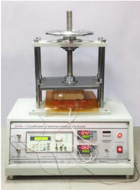
Figure 45: Measuring the thermal conductivity of Mud-Concrete walling material
