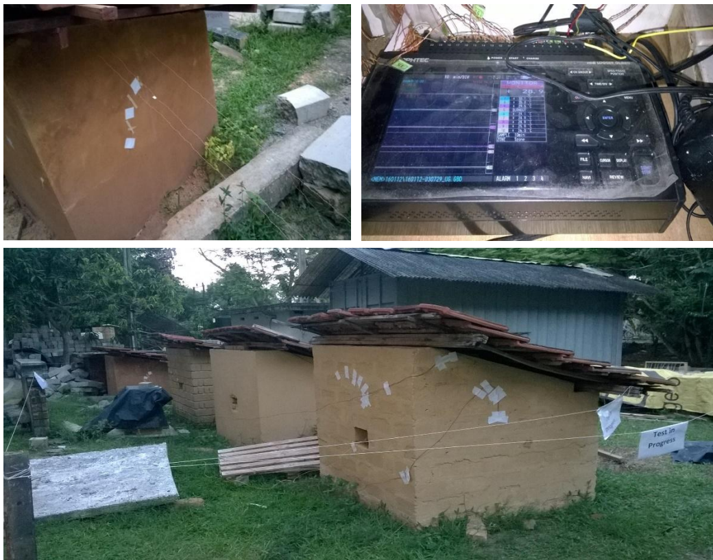
Figure 100: Thermal data measured using GL 820 Midi - data logger and thermo-couples
