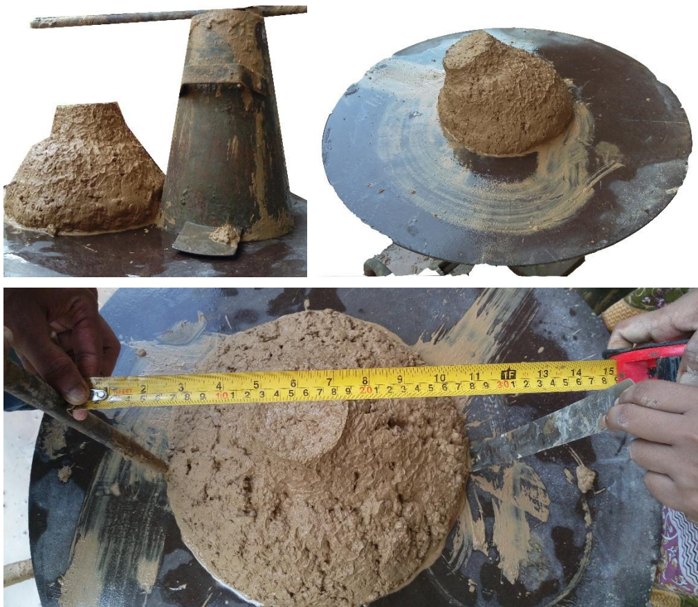
Figure 11: The MC mix has not spread at once due to the cohesiveness of the material.
