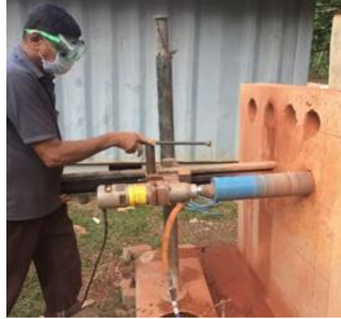
Figure 81: Obtaining MC core samples
