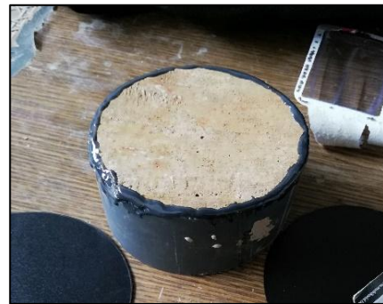
Figure 43: MC sample was fixed and sealed to a PVC cup using epoxy resin
