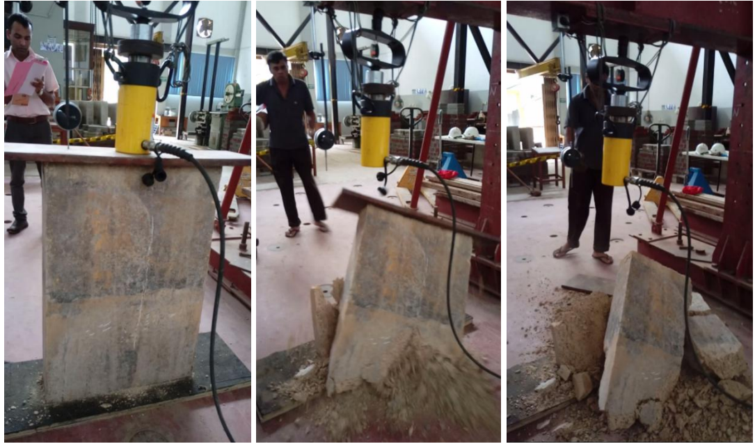
Figure 93: Conducting the load-testing
