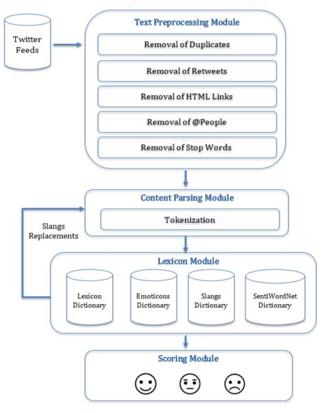
Figure 5.1: High Level Solution Diagram
