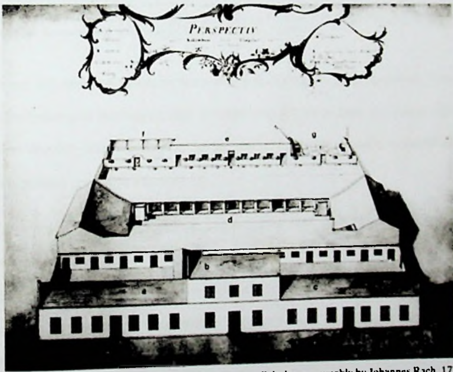
Figure 1. Front view of the Dutch hospital in Colombo. Painting presumably by Johannes Rach, 1771. Koninklijk Instituut voor Taal-, Land- en Volkenkunde, Leiden. A. chief surgeon's residence; B. pharmacy; C. apothecary's residence; D. hospital; E. kitchen; F. cattle shed; G. wall.
