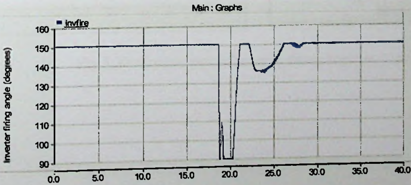
Fig 5.26: inverter firing angle at 3- phase fault
