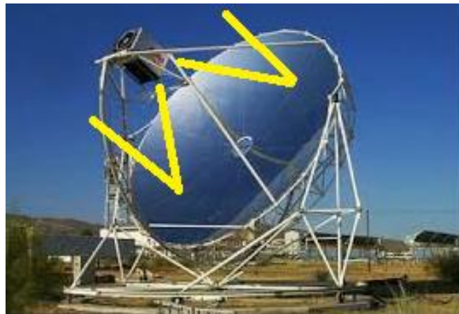
Figure 3.1: Parabolic Dish Collector
