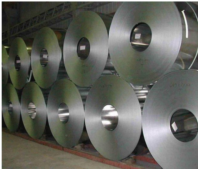
Figure 2.2: Silicon steel mother coils
