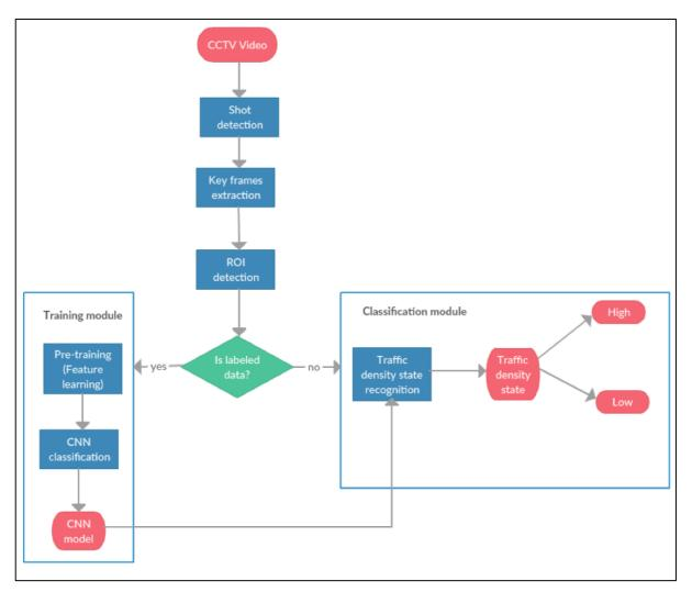
Figure 5.2: Design for traffic density recognition
