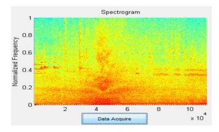
Figure 2.4: Spectrogram of low-density traffic (above 40 km/h)
