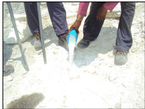
Figure 2.8 Left: Charging of Dynamite with ED (Primer)
