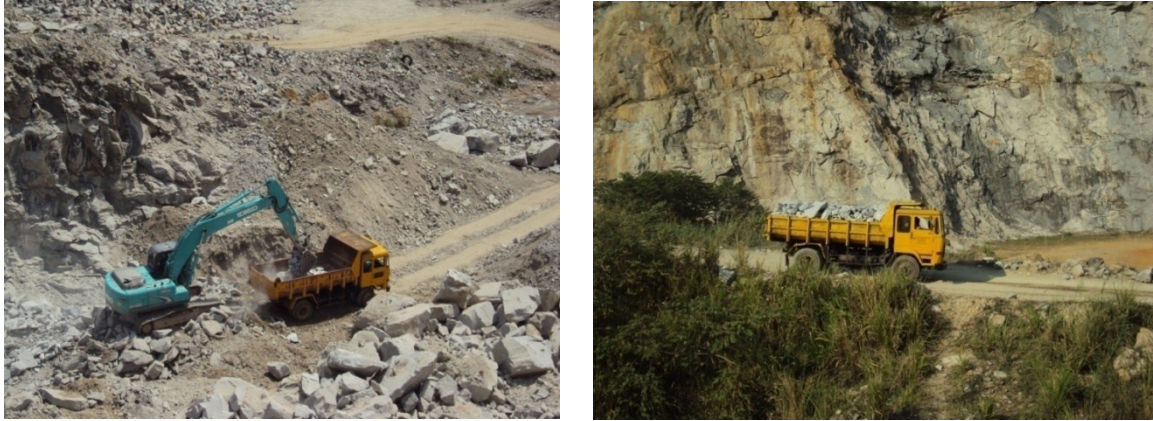
Figure 2.12 Left: Loading to Dump Trucks Right: Material Transportation to Processing or Direct Customers
