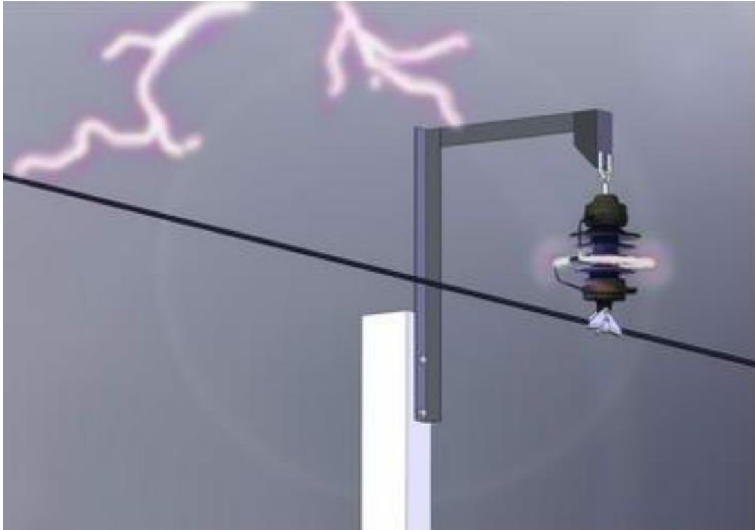
Figure 3.13 MCIA based on a porcelain rod insulator used in 3 kV DC railway overhead contact systems
