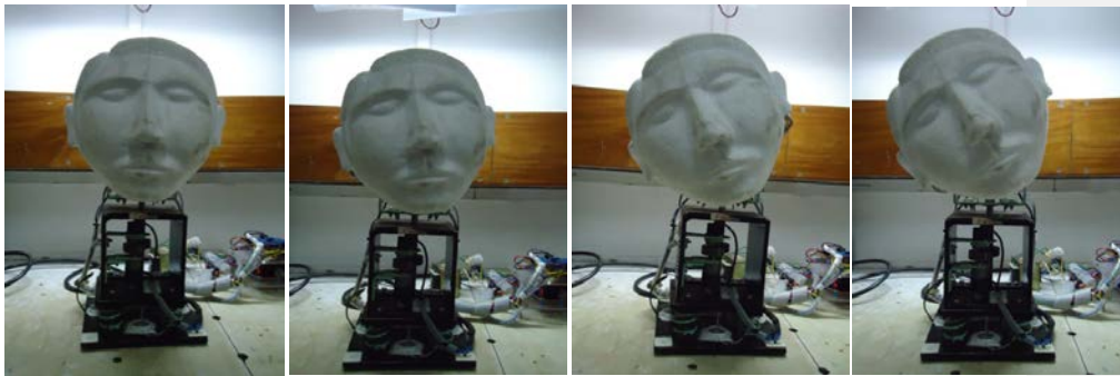
Fig 2.17.(a): Rolling movement of the robot head with face
