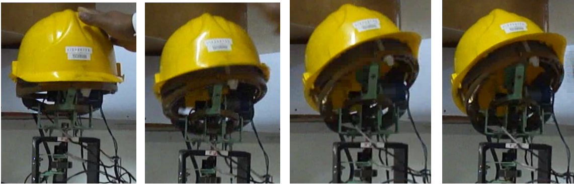
Fig 3.25: Movement of robot head for 0 < \theta < 45 deg
