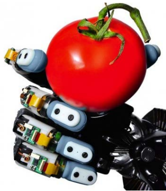
Fig 1.8: Tactile force sensing suite for robot hand
