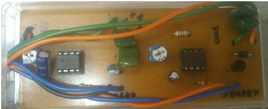
Fig 3.2: PCB designed for force sensing circuit
