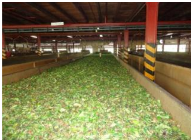
Figure 2.4: Withering process done through troughs
