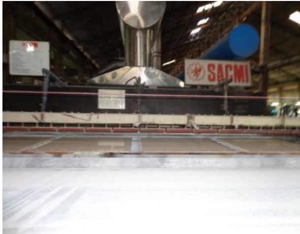
Figure 2.17: Firing process is done in the kiln
