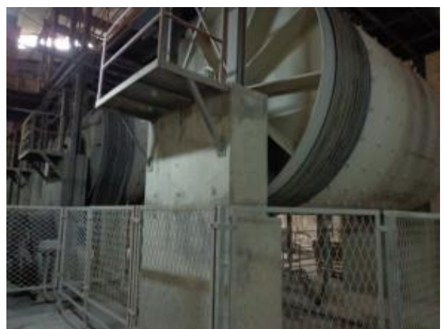
Figure 2.12: Milling process done through ball mills
