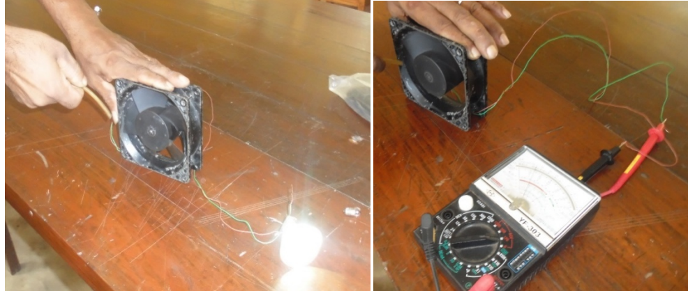
Fig 4.5 Testing the turbine and alternator
