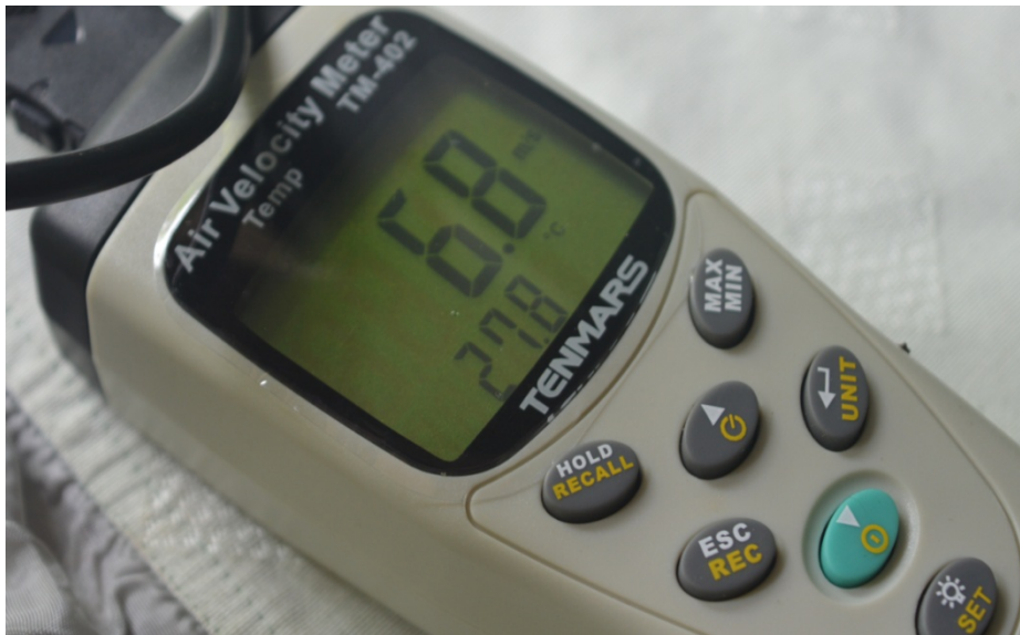
Fig 4.15 Air flow rate testing 2
