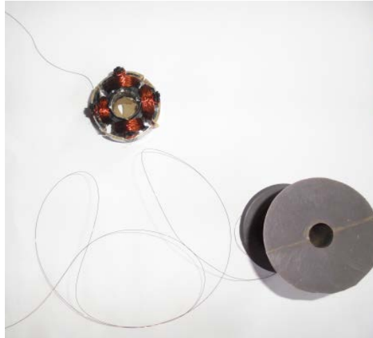
Fig 3.14 Preparing armature of alternator of model generator.
