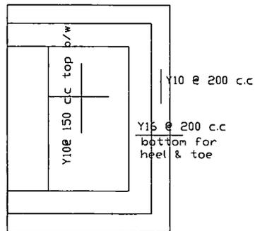
Fig 3.12:Base slab reinforcement arrangement
