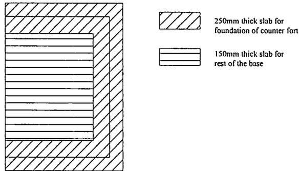
Fig 3.11:Base slab arrangement
