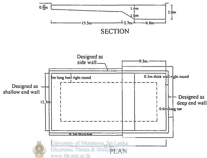
Fig 3.6: Plan and section of conventional swimming pool with a deep end
