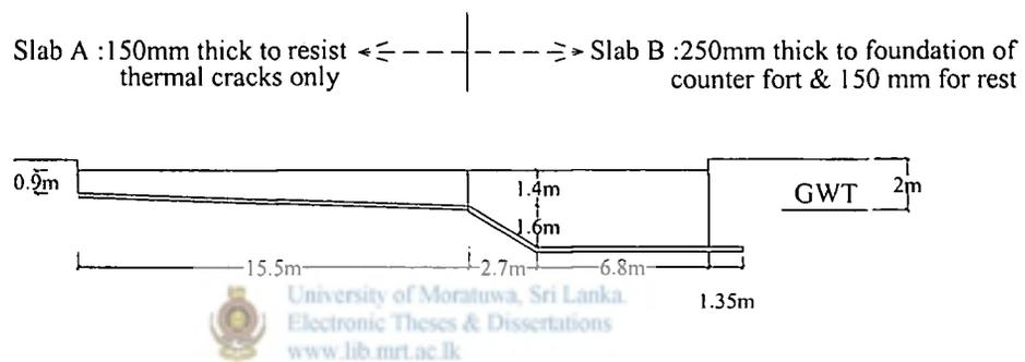
Fig 3.10: Section of pool showing slab thicknesses for design
