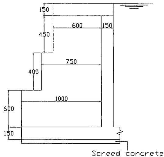
Fig 3.5:Section of wall of 1.6m deep
