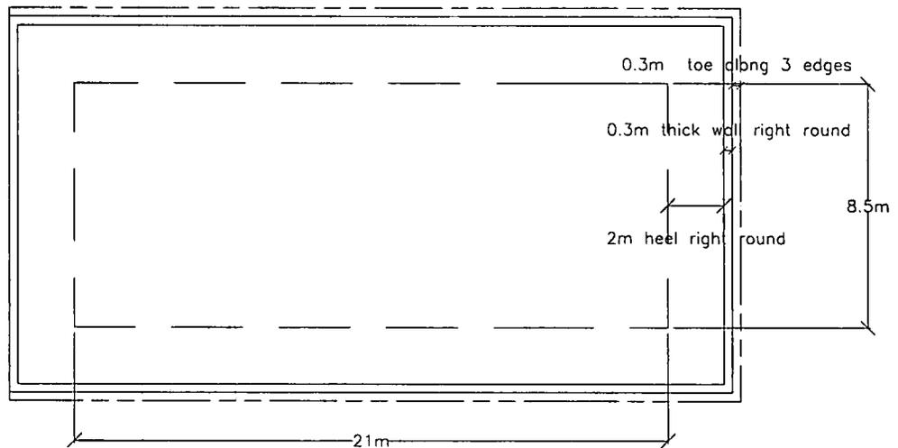
Fig 3.3:Arrangement used for the study
