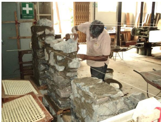
Figure 4.1: (a) – Preparing samples for Flexural Strength Test
