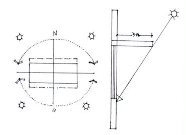
Figure 8 – Horizontal devices to stop direct sun onto the north facing walls
