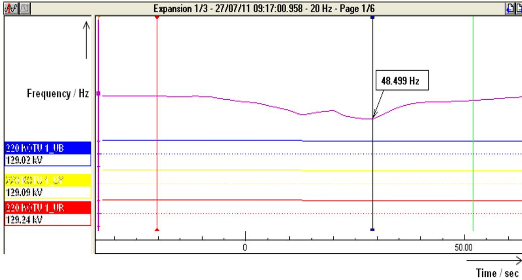
Figure 2.3 – System Frequency variation on 27<sup>th</sup> of July 2011 at 09.17 AM
