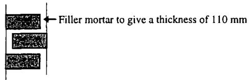
Figure 6.1: Bond arrangement for 110 mm thick brick walls
