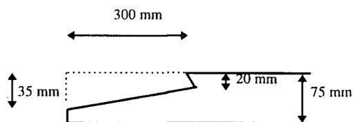
Figure 6.4: Dimensions to calculate the volume of insitu cast concrete over block walls
