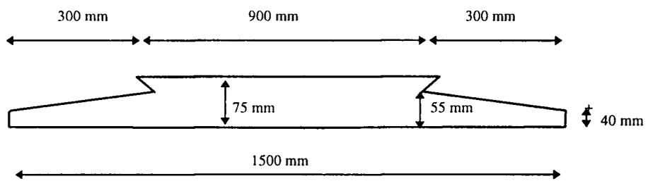
Figure 6.2: Dimensions of the precast panel of width 300 mm
