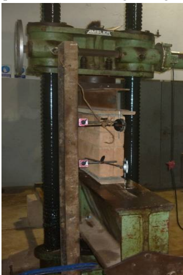
Figure 2 Testing of wall panel
