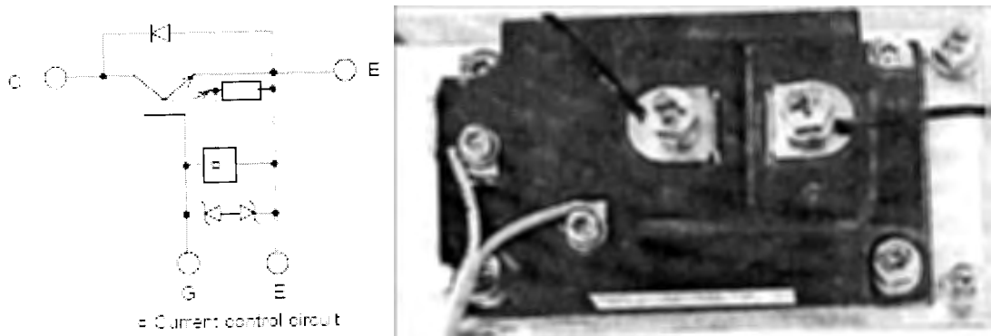
Fig-6.4: Equivalent Circuit Schematic and Actual Figure of the IGBT Module
